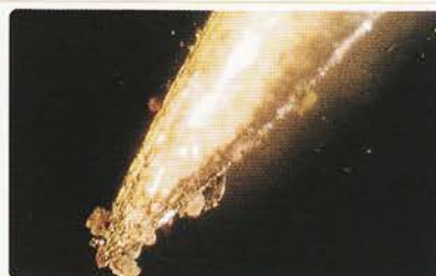
Contaminants attracted to the end of magnetized needle in the oil on a slide glass
